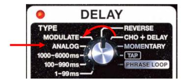
2. Set the DELAY Control knobs to an appropriate setting.
